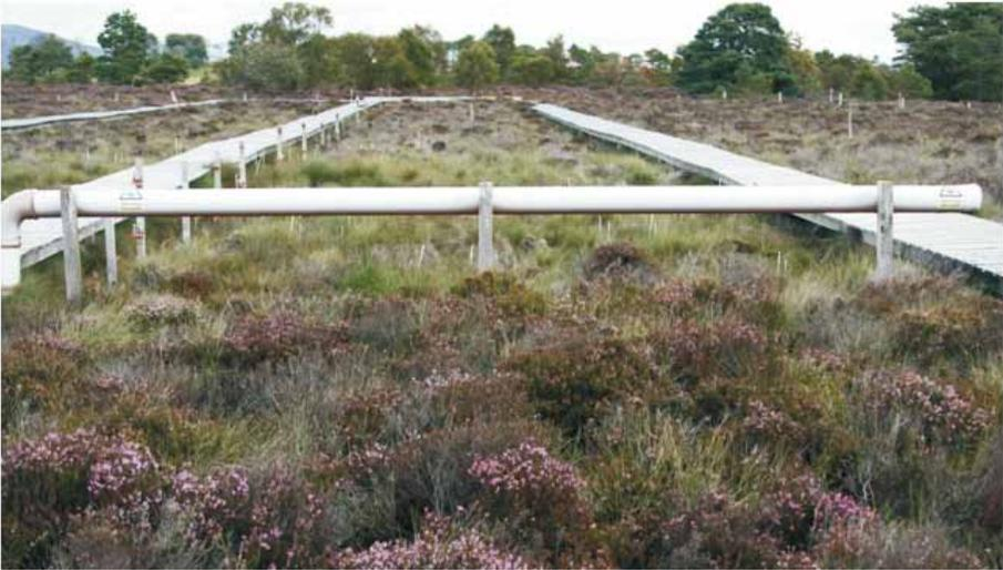
Figure 5.22: Photograph (taken on 27/08/09) looking downwind of the 60m ammonia free air release transect at Whim Bog, a lowland raised bog in the Scottish Borders. The photo shows the undamaged vegetation upwind of the 6m release pipe and the change in vegetation with the loss of *Calluna vulgaris*, *Sphagnum* spp. and *Cladonia portentosa* up to 24m downwind of the  $\text{NH}_3$  release point, which is now dominated by *Eriophorum vaginatum*. © Ian Leith
